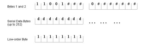
Where the five high-order bits are set to 1-1-0-0-1, denoting the start of new serial data. The high-order bit of byte 2 is set to 0. The 10-bit index of the signal (identified by # signs) is spread out over bytes 1 and 2, with leading zeros used as fills. This is followed by up to 252 bytes of serial data (identified by the "d" letters). Finally, the low-order byte is set to FFh (binary 1111 1111) denoting the end of the serial data.
